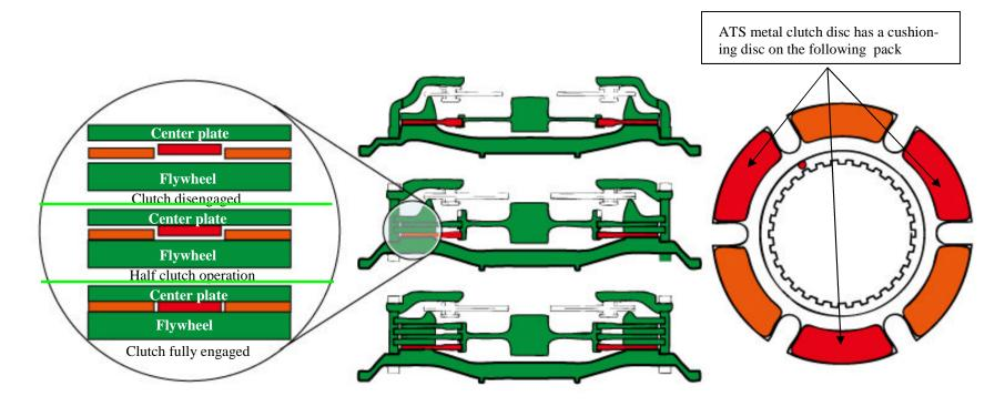
Very smooth half clutch and engagement from ATS metal clutch cushioning disc design !!
